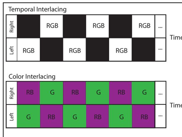
**Figure 1.** Temporal interlacing vs color interlacing. The upper panel represents conventional temporal interlacing and the lower panel color interlacing. In temporal interlacing, full RGB images are presented alternately to the two eyes. In color interlacing, the green channel (G) is presented to the left eye at the same moment that the red and blue channels (R and B) are presented to the right eye. The channels are reversed in the subsequent sub-frame.
