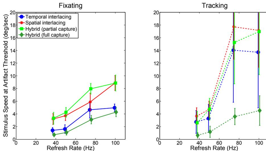
Figure 4. Motion artifacts in 4 display protocols. The stimulus speed at the artifact threshold is plotted as a function of refresh rate. Greater values on the ordinate axis indicate smoother motion. For the fixating case, motion looks markedly worse in the hybrid full capture and temporal interlacing protocols, as predicted. For the tracking case, the hybrid full capture had the most pronounced motion artifacts.
