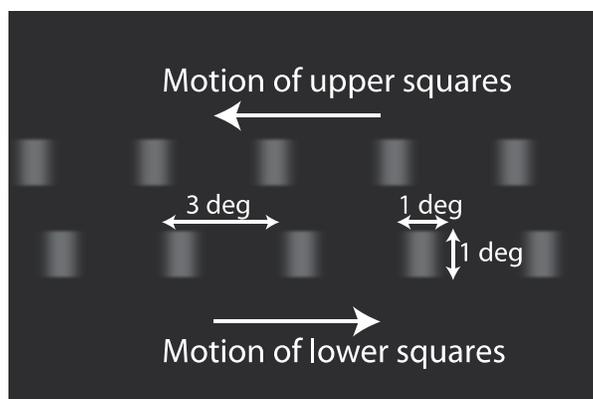
Figure 8. Illustration of the experimental stimulus used to measure depth distortion. Two groups of bars moved horizontally in opposite directions. If there was any depth distortion, one group appeared to be closer while the other appeared farther than the display surface. The task was to choose which group appeared closer (2 alternative forced choice).
