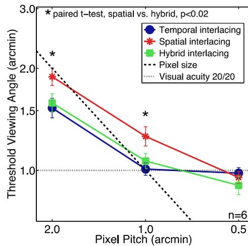
Figure 7. Effective resolution of three display protocols. Threshold viewing angle, or the minimum stroke width resolvable at threshold performance level, is plotted as a function of pixel pitch. When pixels are large (2 arcmin), temporal and hybrid protocols have improved resolution compared to spatial interlacing (paired t-test,  $p < 0.02$ ). When pixels are small (0.5 arcmin), there are no
