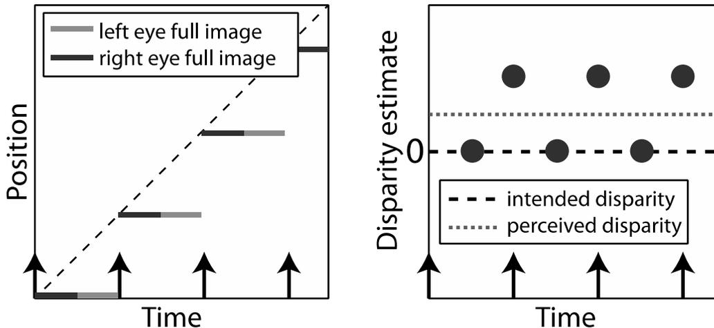
Figure 2. Left: Temporally interlaced stereo presentation. Right and left eye images are captured simultaneously but displayed in alternation. Right: The visual system attempts to match left and right eye images, but there is inherent ambiguity in the match, resulting in false matches 50% of the time. The perceived disparity is shifted from the intended disparity.
