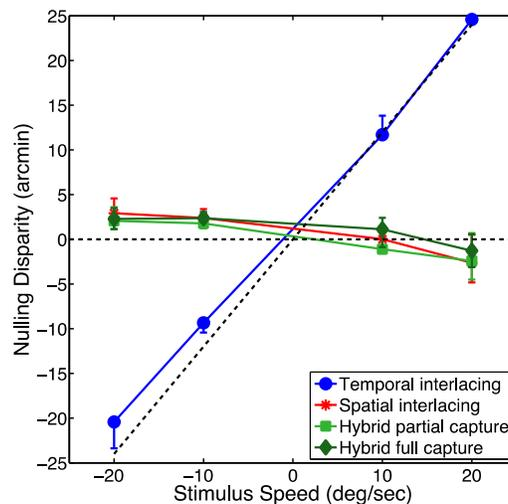
Figure 9. Plotted is the nulling disparity necessary to make the right- and left-moving objects appear at the same depth for a given stimulus speed. The diagonal dotted black line is the prediction based on equation 1. Spatial and hybrid interlacing appear to have little depth distortion, and temporal interlacing has depth distortion in line with predictions.
