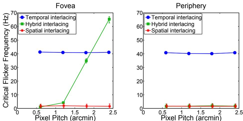
Figure 5. Critical flicker frequency as a function of pixel pitch. Plotted above are flicker thresholds for spatial, temporal, and hybrid interlacing, pooled across all subjects. For temporal and spatial interlacing, thresholds do not change as a function of pixel size. For hybrid interlacing, flicker becomes noticeable when pixels are large but is absent when pixels are small.
