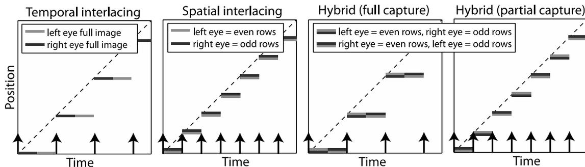
Figure 1. Four stereoscopic 3D display protocols. Arrows indicate the times at which content is captured. Note that spatial interlacing and hybrid (partial capture) allow for twice the capture rate of temporal interlacing, which should create smoother looking motion.
